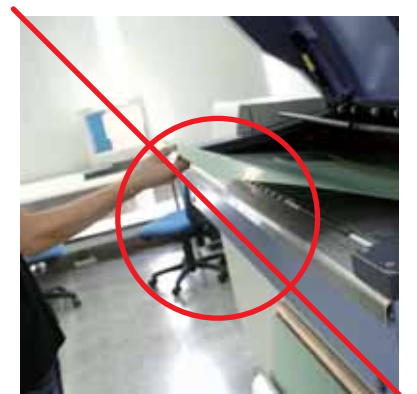
When loading plates, ensure the product is well supported to avoid damage.
